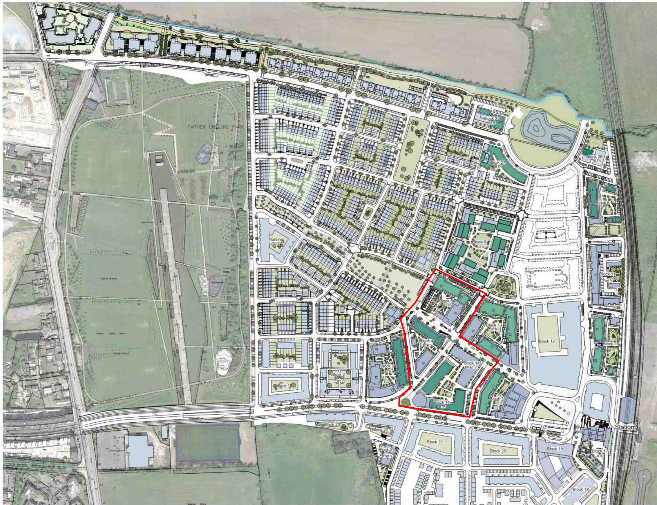
Landscape Architect's drawing showing living roofs and landscaped podium courtyards across the application
