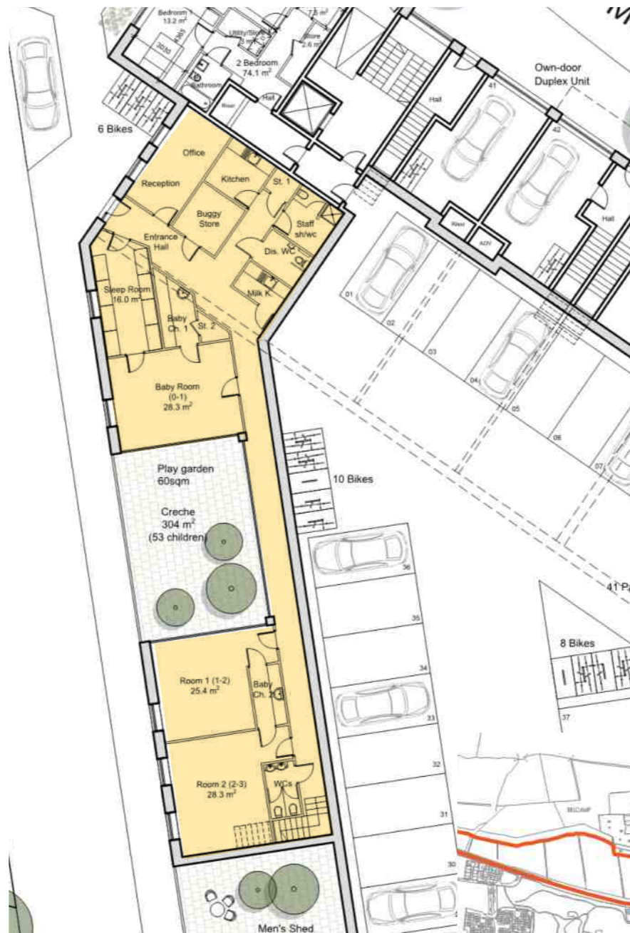
Layout of creche in Block 4, showing spaces laid out over two floors with rooms arranged around an external play space at ground floor
